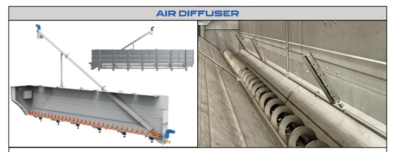
The combined effect of the micro and macro air bubbles creates a deposition effect of the sand particles. The lower horizontal conveyor auger conveys the deposited sands up to the extraction area, where the inclined screw extracts and discharge the material. After the treatment, the sand-free organics can be introduced into the digester.
