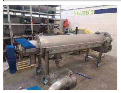
Primary sludge is pumped passing through a perforated drum, which by a screw that catch and push out the screenings cleans the inlet flow keeping it pressurized. In the last stage of this process is a cone which pneumatically regulates the counter thrust in order to hold the pressure inside the unit.
