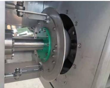
A self-cleaning screw combined with motorized washing which, running through the entire drum, guarantees cleaning and therefore maximum efficiency.
