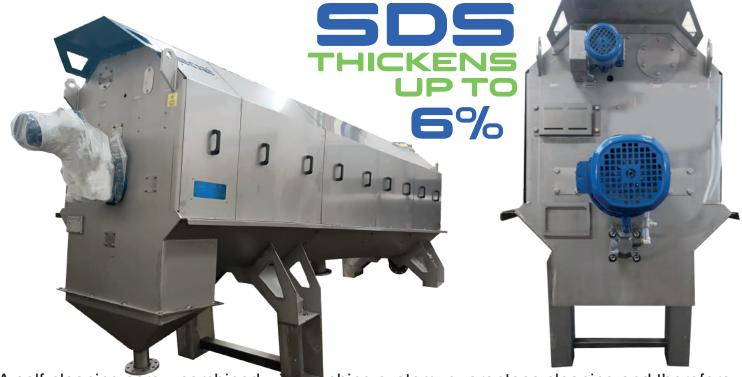
A self-cleaning screw combined with ashing system, guarantees cleaning and therefore maximum efficiency.
